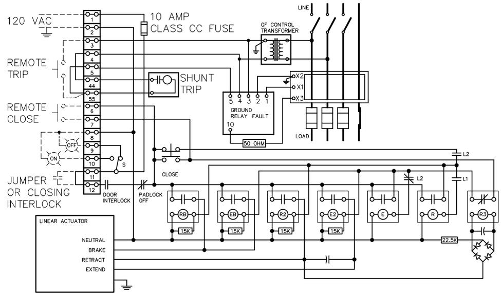
**MST WIRING WITH INTEGRAL GROUND FAULT**
