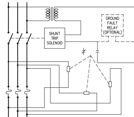
**BLOWN FUSE DETECTOR WITH SHUNT TRIP OPERATOR**
